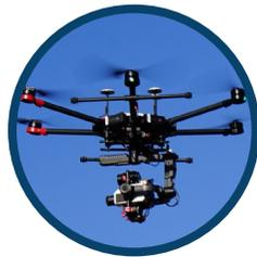
**Avitas** | OGI cameras affixed to drones capture up-close videos of facility emissions. The flight path is pre-planned to visit and inspect all potential sources of emissions in an efficient manner. The final product directly links the emission to a piece of equipment and includes video support. Product is approved for EPA OOOOa inspections. TRP used Avitas across nine of our largest producing facilities on Nov. 18.
